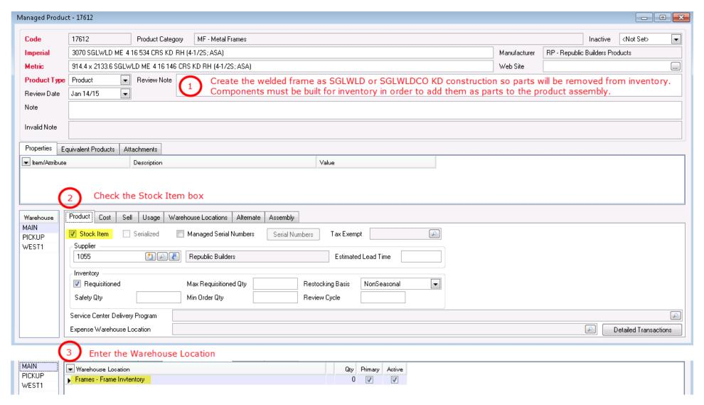
After saving the managed product just built click on the Product Assembly tab to add the components and labor for the shop welded frame.
